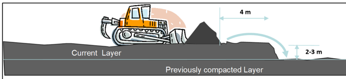
Figure 2: Operating methodology for dumping and dozing of Rock Fill Material
