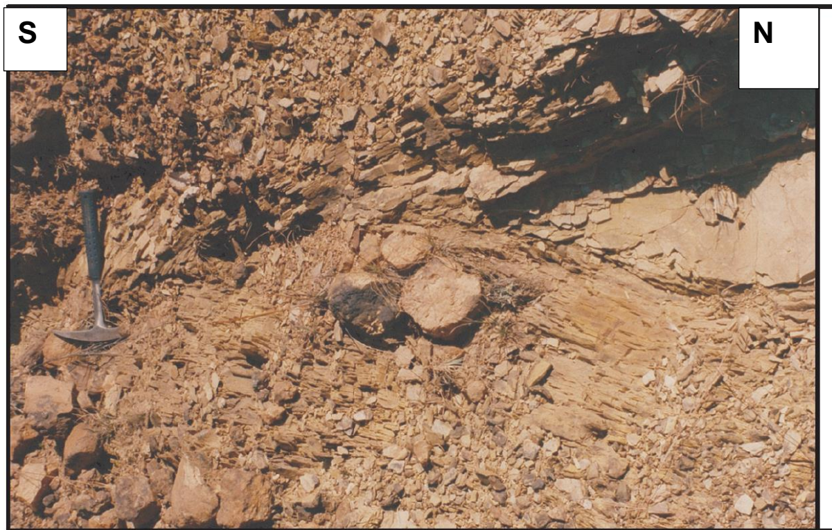
Fig. A3: Tight, probably faulted and overturned fold in slate (view to west), lower Timeball Hill Formation near Glen Africa Country Lodge (cf. Figure 2); bedding dips: upper limb 57^\circ to SE, lower limb 22^\circ to ENE (Ingram et al., 2000).
