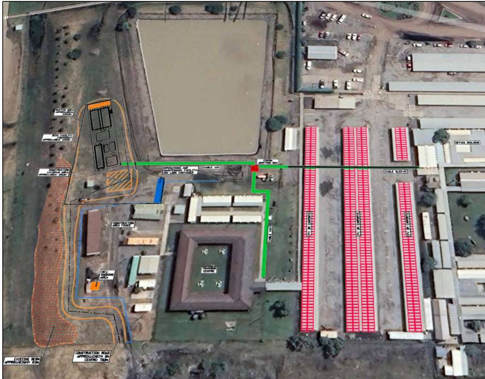
Figure 4: Site Layout for the proposed Tharisa BESS Development
