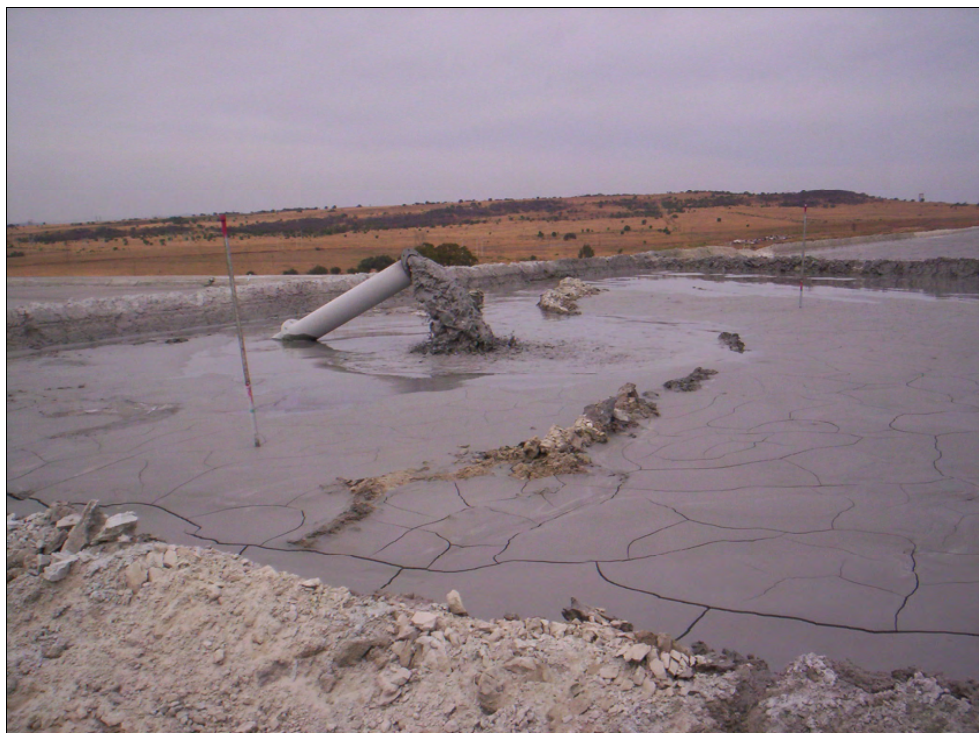
FIGURE 1: DEPOSITION OF FRESH TAILINGS AT THE OPERATIONAL TSF
