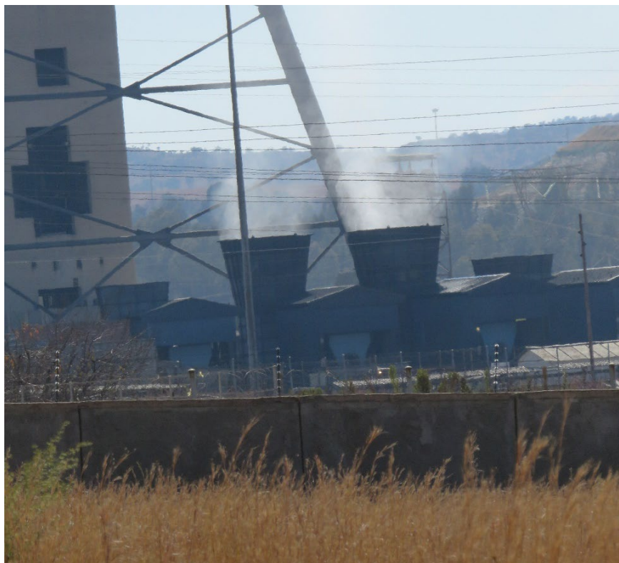
Figure 2.8 Air released from the ventilation shafts at the surface at the Twin Shaft Complex of the South Deep Gold Mine.
